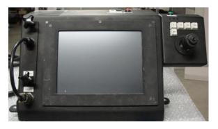
Command pulpit equipped with touch screen computer / monitor and joystick with push button; the pulpit contains a removable hard disk and the service box.
